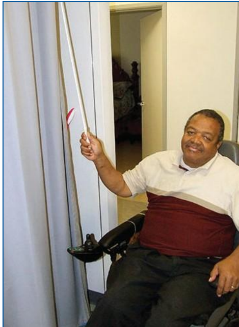
F Closets use curtains with pull-rods
